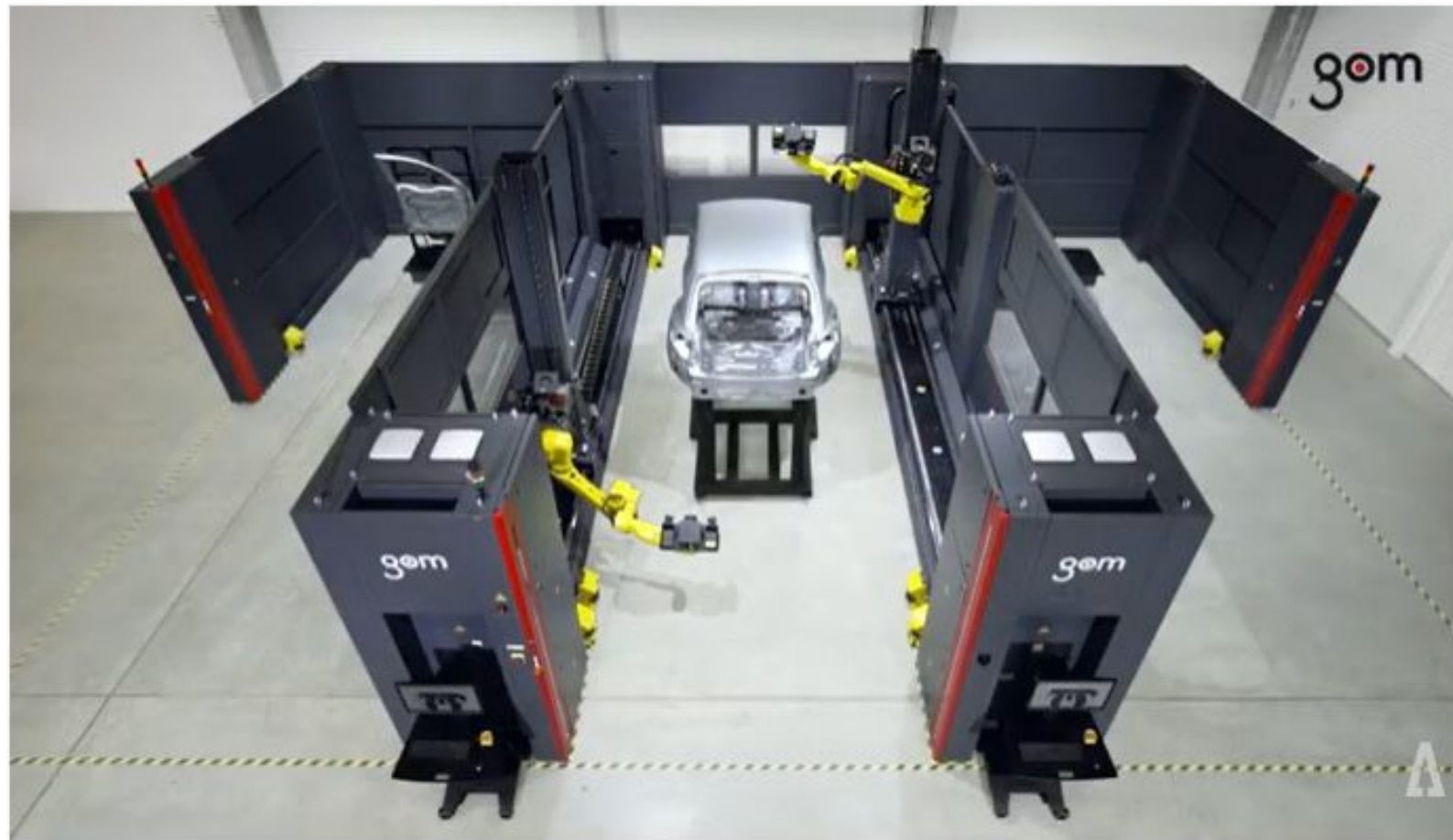
3D Laser Scanner Measures Automotive Car Body in Inspection Cell
